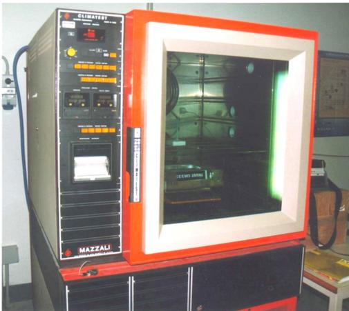
Fig. A-1: The climatic chamber employed for the aging process and the thermal expansion coefficient measurements.
