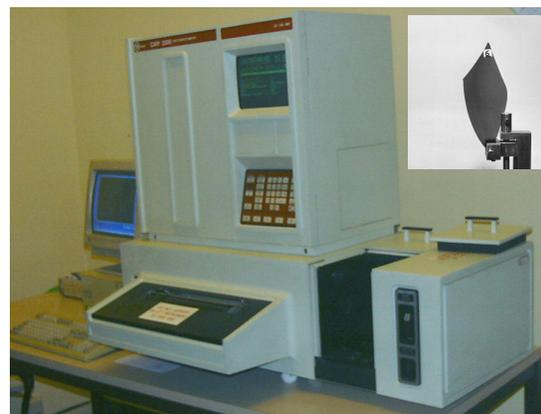
Fig. A-2: The spectrophotometer Cary 2300 employed for the optical properties measurements; in the box sample No. 6 is illustrated.
