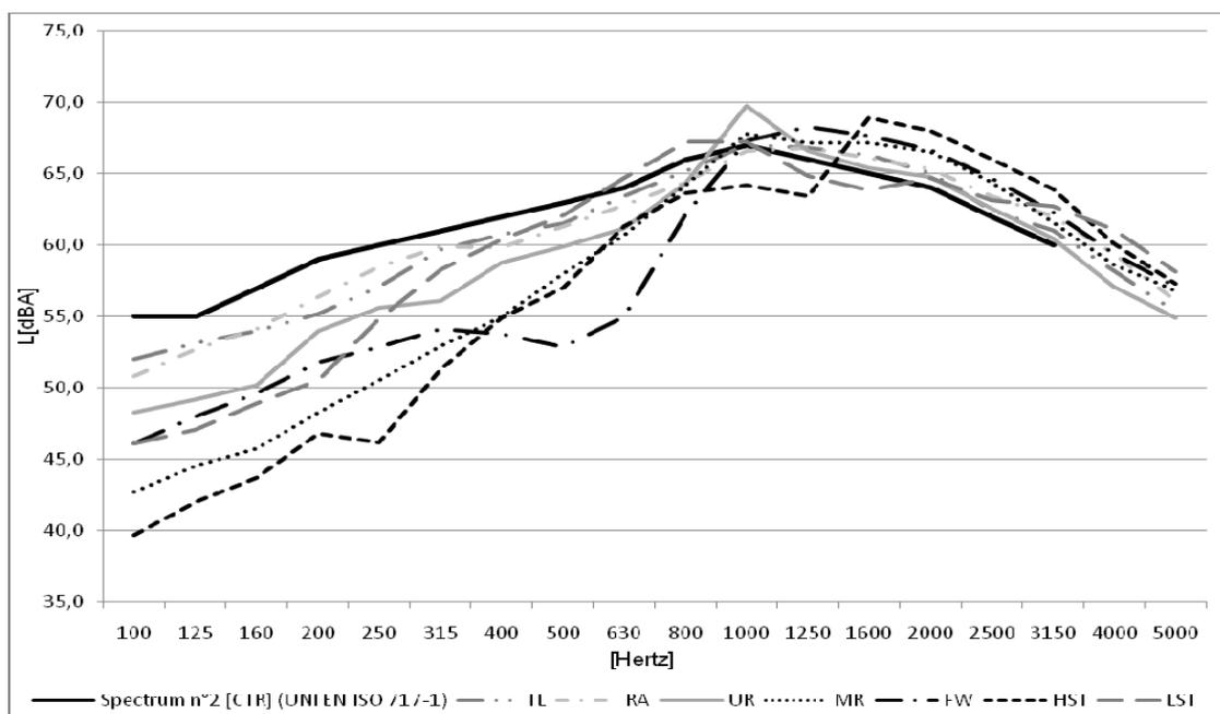
**Figure 2:** Registered noise spectra compared to Ctr spectrum (ISO 717-1).
