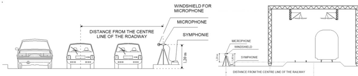
**Figure 1:** Sampling of traffic and train noise spectra
