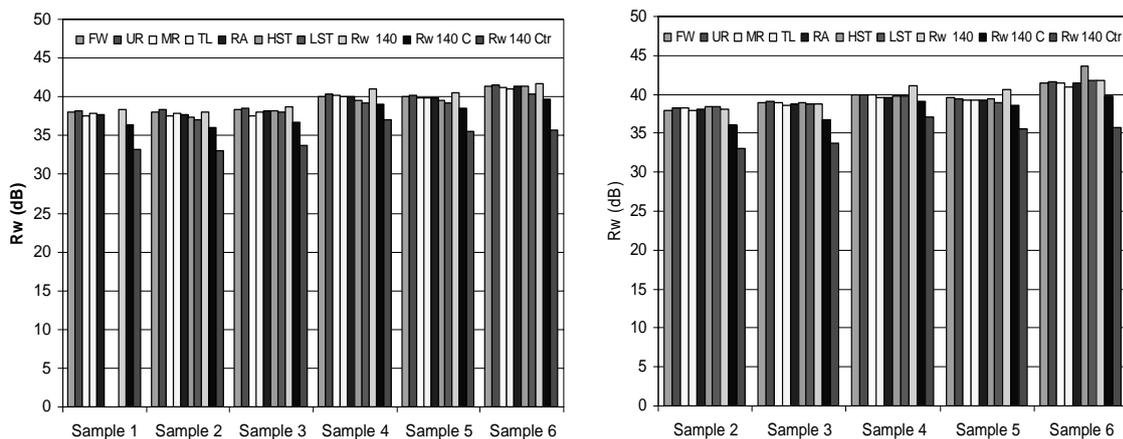
**Figure 3:**  $R_w$  evaluated with different spectra, with ISO 140-3 and corrected with C and Ctr for the different samples; A) Signal; B) MGS.
