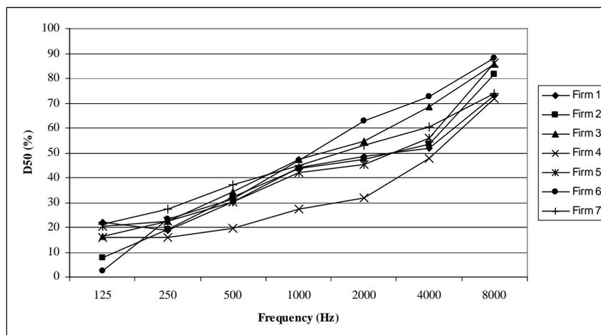
Figure 4 – Measured  $D_{50}$  values for the seven different electro-acoustic systems
