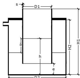
**Figure 8:** Schematic diagram of gas-meter
