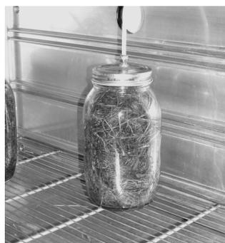
**Figure 2:** Anaerobic glass vessel reactors in climatic chamber
