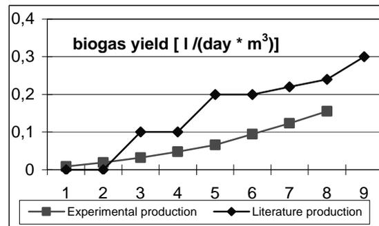
**Figure 7:** Comparison between experimental biogas production and the Literature values.
