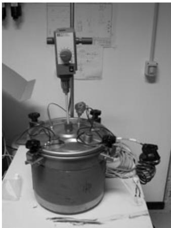
**Figure 6:** Batch digester equipped with probes, heating and stirring systems.
