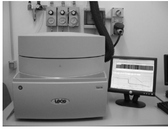
Figure 2: TGA 701 LECO for Proximate Analysis
